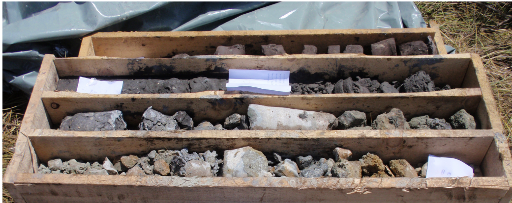
Figure 4. Samples of coal ash and slag from exploratory boreholes.
